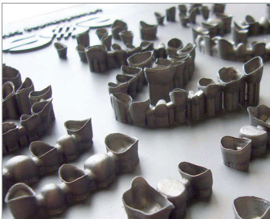
Figure 1: A batch of laser-sintered copings and bridges, made of cobalt chrome.
