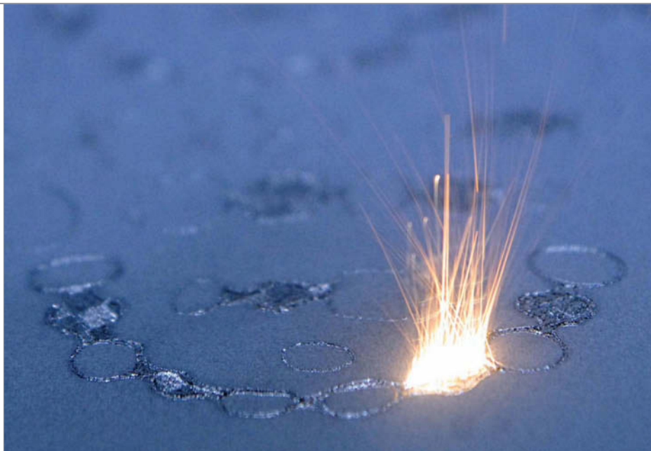
< Figure 2: An image of dental copings and bridges being laser-sintered.
